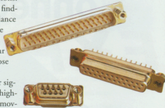
Figure 2. These pressfit vertical plug and socket D-subminiature connectors manufactured by ERNI Components Inc. are designed for the demanding requirements of the backplane market. They feature tin-plated steel shells and PBT insulators and are available in nine-, 15-, 25-, 37- and 50-pin configurations with preinstalled stand-offs and other mounting hardware.
